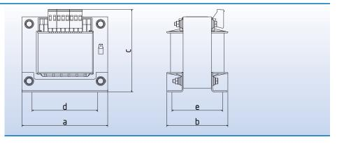
Single-phase autotransformers according to VDE 0570 part 2-13, EN 61558-2-13
