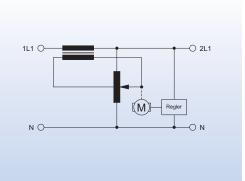
Single-phase and 3-phase voltage stabiliser according to VDE 0552/69
