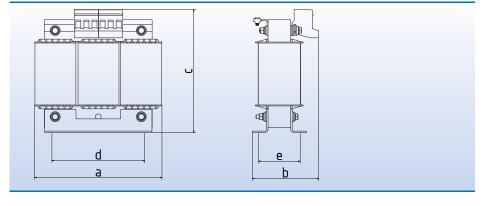
Three-phase line chokes according to VDE 0570 part 2-20
