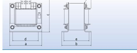
Single-phase double line chokes according to VDE 0570 part 2-20
