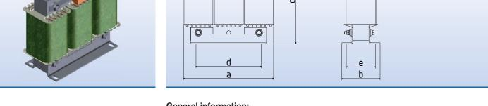
Three-phase filter circuit chokes according to VDE 0570 part 2-20
